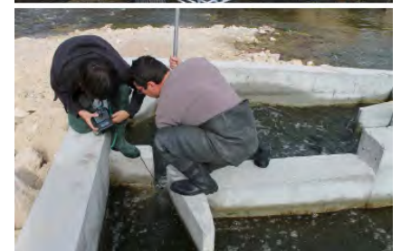
Figure 12. Different assessment procedures for fish-ways: a) Stopping water flow in the fish ladder and capturing fish b) Trapping via orifices and c) Hydraulic assessment
