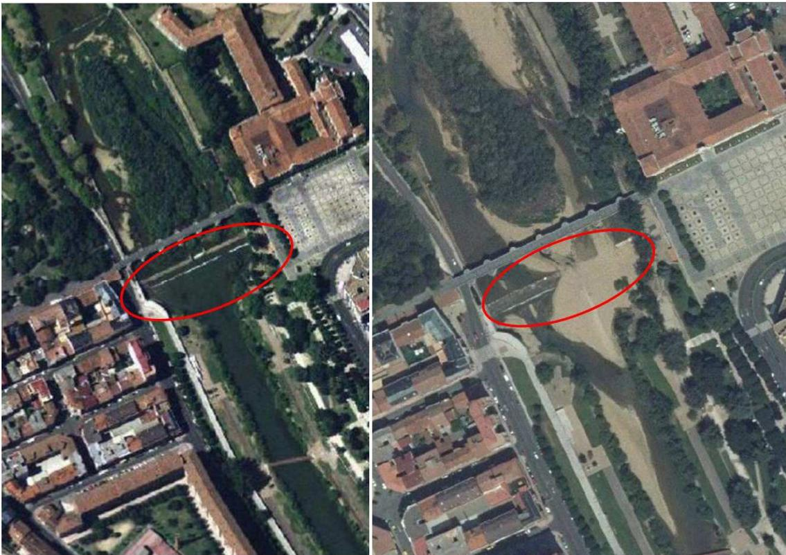
Figure 27. Image of the Bernesga River before (left side) and after (right side) the works of removal.
