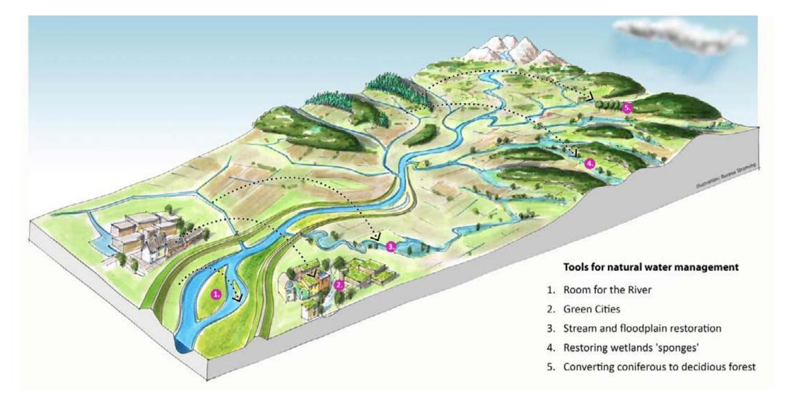
*Figure 1. Tools for natural water management. In a basin approach a broad array of measures is taken which together – not in isolation – generate the desired effect: less peak flooding, shorter periods of drought.*
