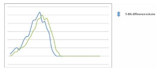
Figure 15. Synthetic discharge hydrograph based on the travel time in the Prüm catchment for situations without (blue line) and with (green line) sponge restoration. Y-axis = discharge X-axis = time. Development of sponges would lead to 5-8% lower peak discharges.
