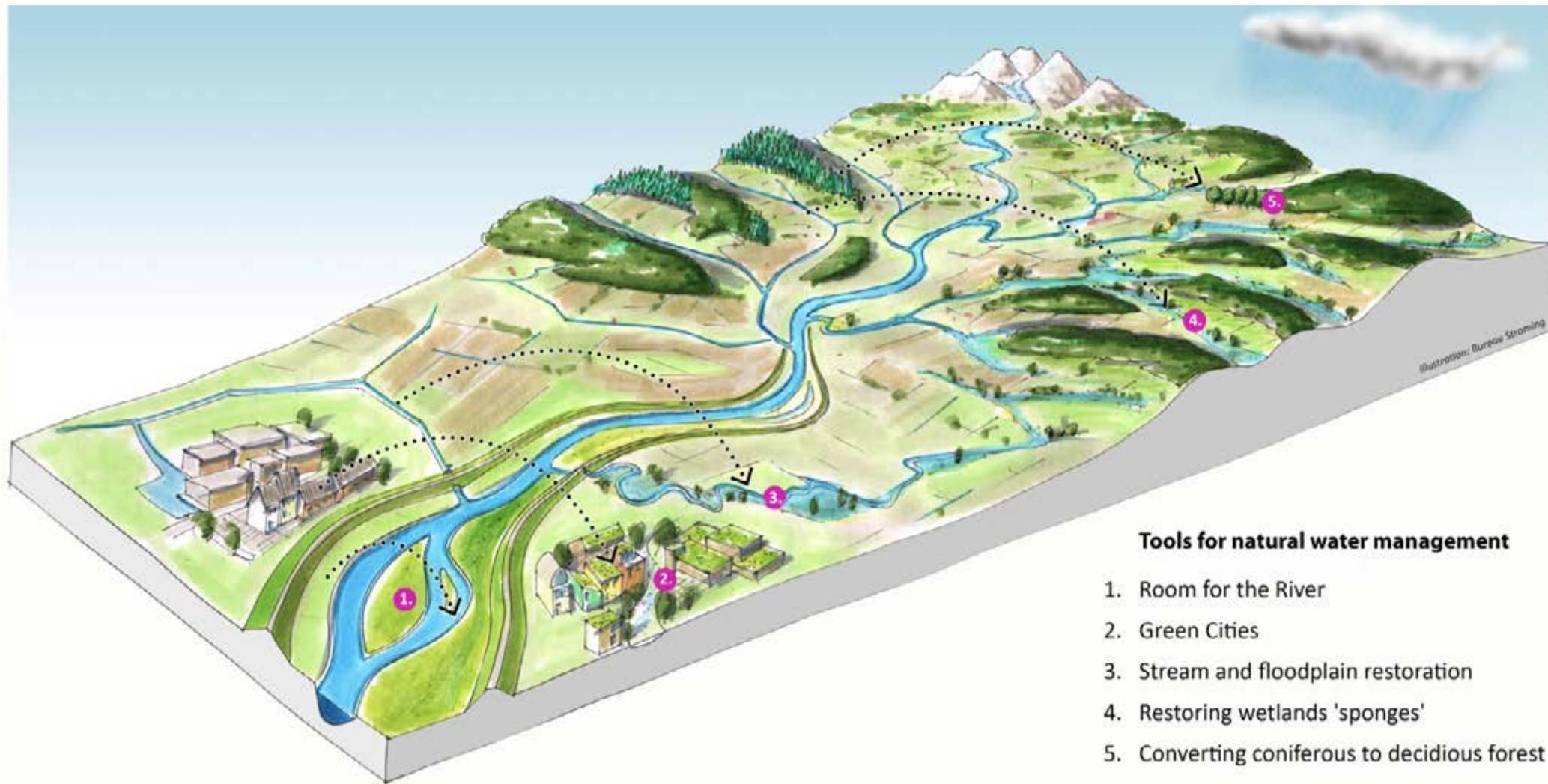
Figure 1. Tools for natural water management. In a basin approach a broad array of measures is taken which together – not in isolation – generate the desired effect: less peak flooding, shorter periods of drought.
