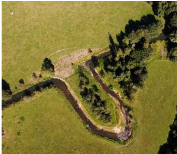
Figure 2. Re-meandering of the Eau Blanche at Boussu-en-Fagne (source: LIFE project «Walphy» Layman's report).
