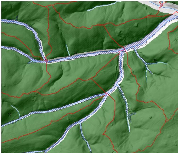
Figure 14. Example of the landscape unit creation technique creating a buffer 10x the width of the channel (white). The pre-determined approximate wetland restoration project areas (blue hatched lines) have been included for reference.
