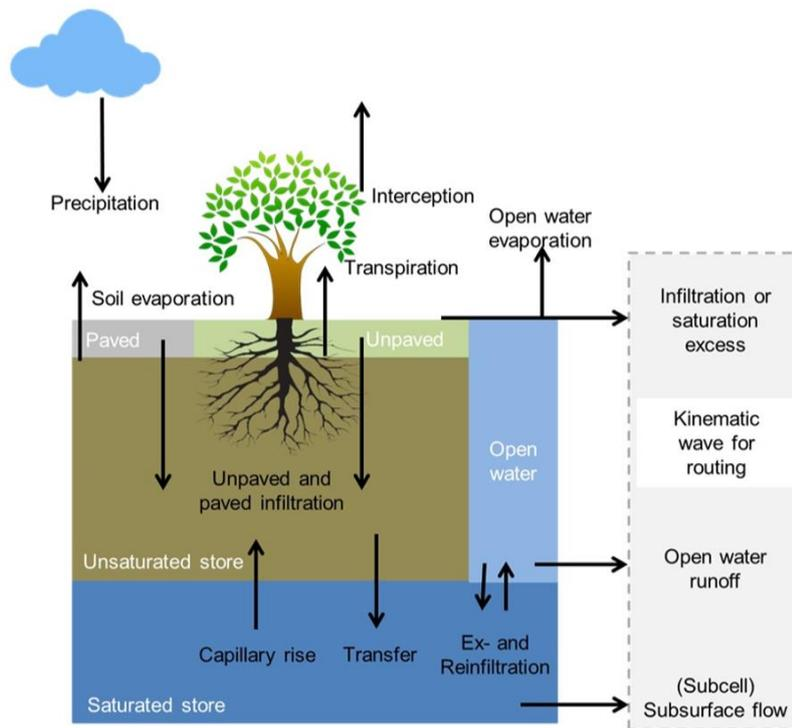
Figure 15. Schematic showing the processes in the WFLOW\_sbm model within each grid cell.
