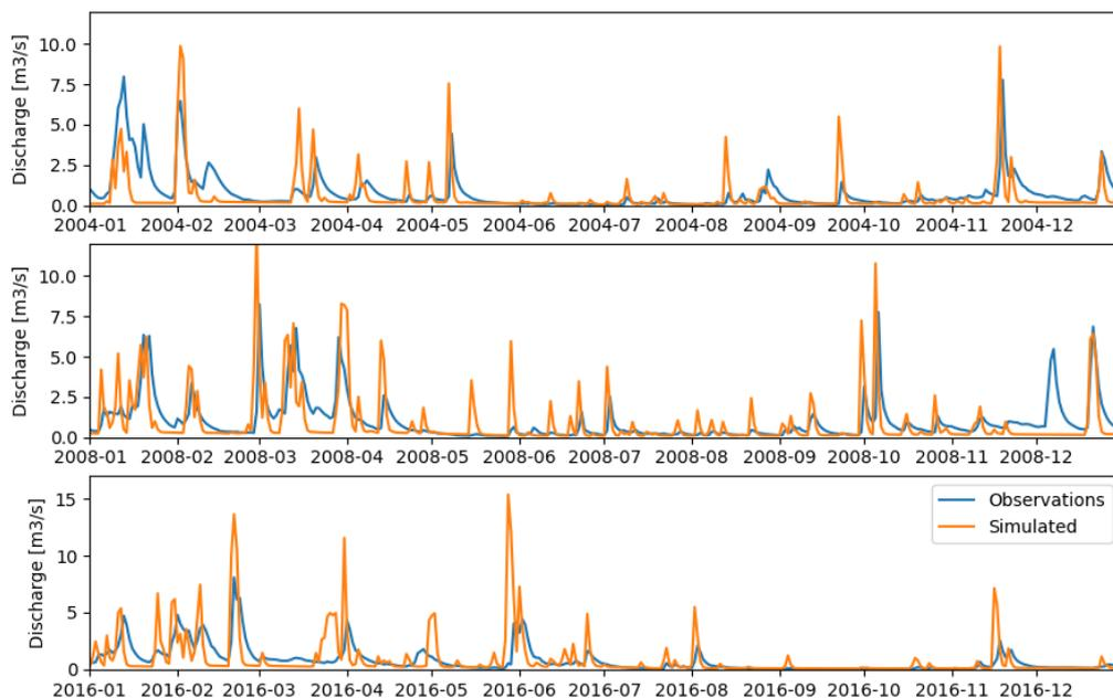
Figure 19. Comparison of measured and SWAT+ modelled discharge for the reference scenario of the Kylldal catchment at Steinebrück outlet for the years 2004, 2008 and 2016.
