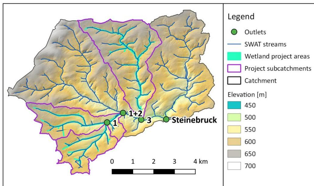
Figure 1. The elevation of the watershed draining to the Steinebrück gauging station and the delineation of the three project subbasins with their outlets. The pre-determined approximate delineation of the wetland project areas is included for reference.
