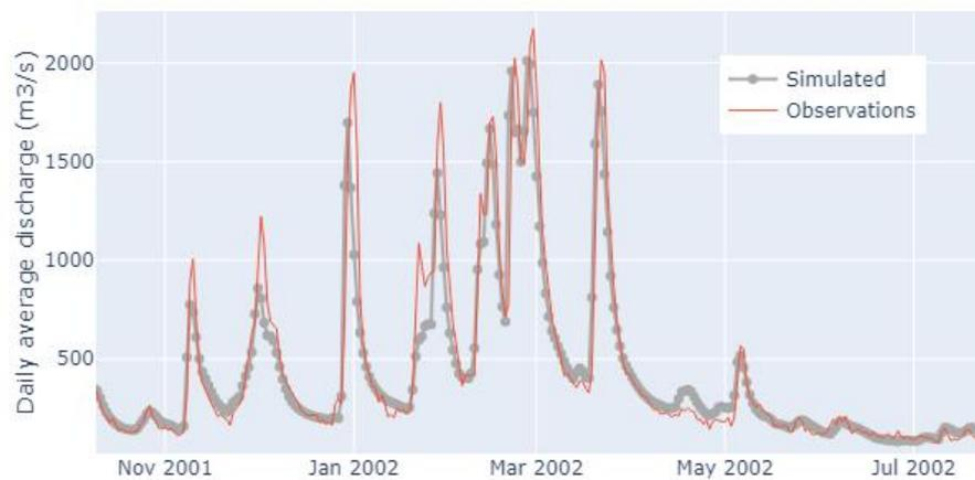
Figure 16. Close-ups of the observed and WFLOW simulated daily average discharge time series at Cochem.
