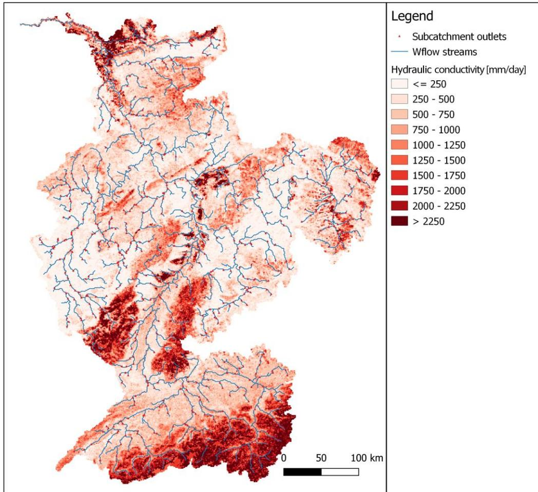
Figure 6. Map showing the  $K_{SAT}$  values in the WFLOW model for the Rhine catchment.
