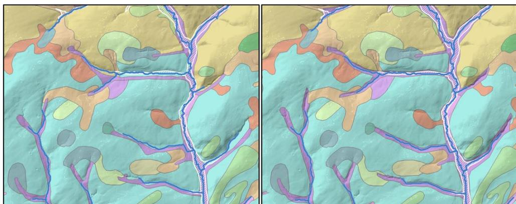
Figure 3. Example of a mismatch between soil type and stream network derived from the DGM1 elevation data (left) and the correction (right). Pink and purple colors are typical valley floor soil types, the white semi-transparent areas are predetermined approximate wetland restoration project areas.
