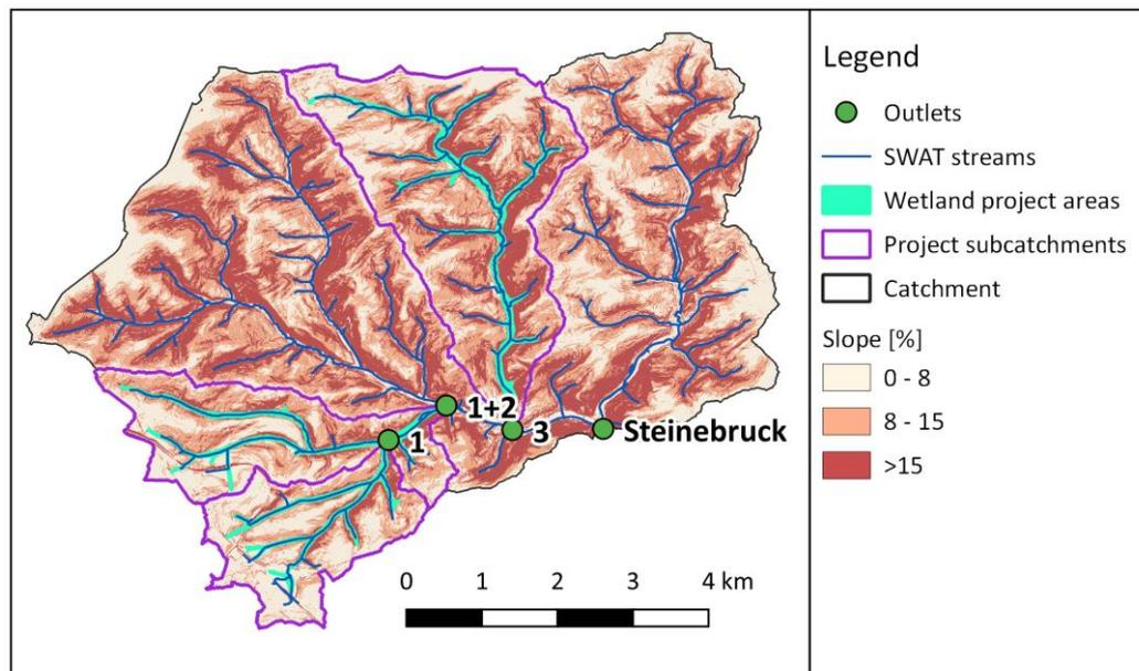
Figure 2. Overview of the slope classes and the project subcatchments, their outlets and the stream network produced by SWAT+. The pre-determined approximate wetland project areas are shown for reference.
