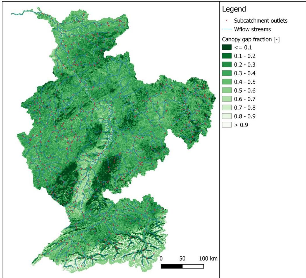
Figure 7. Map showing the canopy gap fraction values in the WFLOW model for the Rhine catchment.
