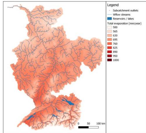
Figure 10. Annual average actual evapotranspiration over the Rhine catchment according to the WFLOW model.
