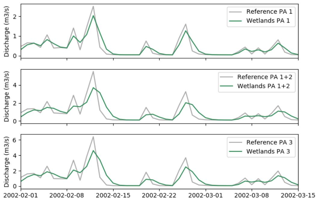
Figure 21. Time series of daily discharge during a winter period with a peak flow event (12-02-2002) for the three project areas in the reference model and the wetland scenario.
