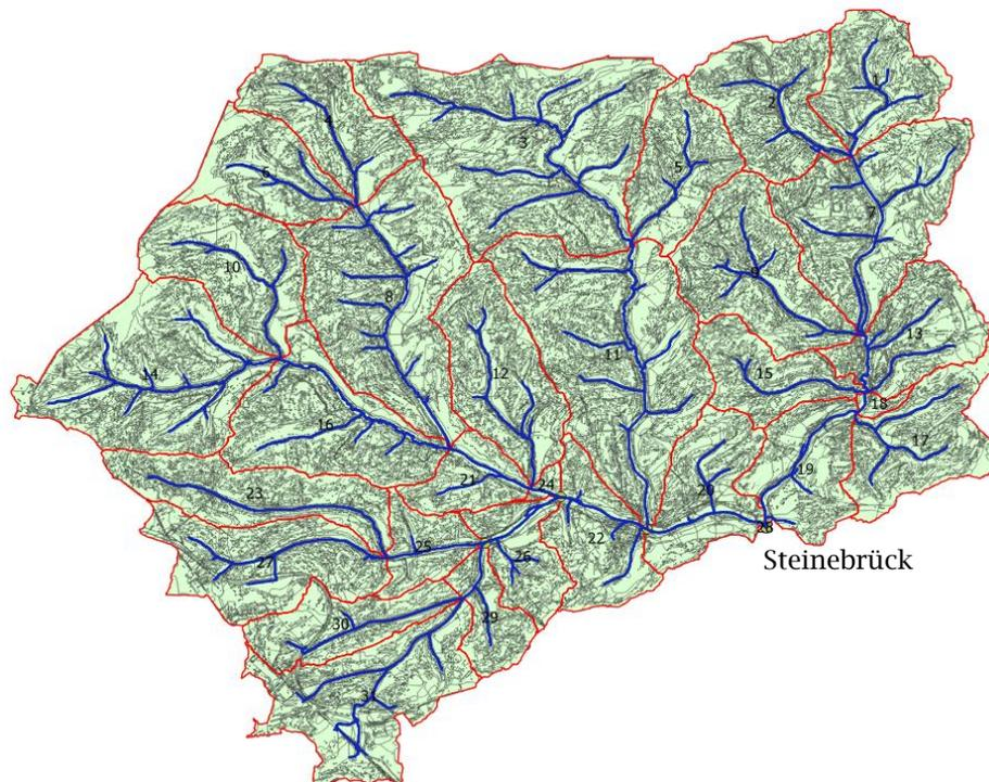
Figure 12. Overview of the 31 subcatchments (demarcated by red lines), 7631 HRUs (grey lines - green background), and 251 interconnected stream channels (blue lines) as defined in the SWAT+ model that make up the Kylldal catchment with the outlet at Steinebrück discharge station.
