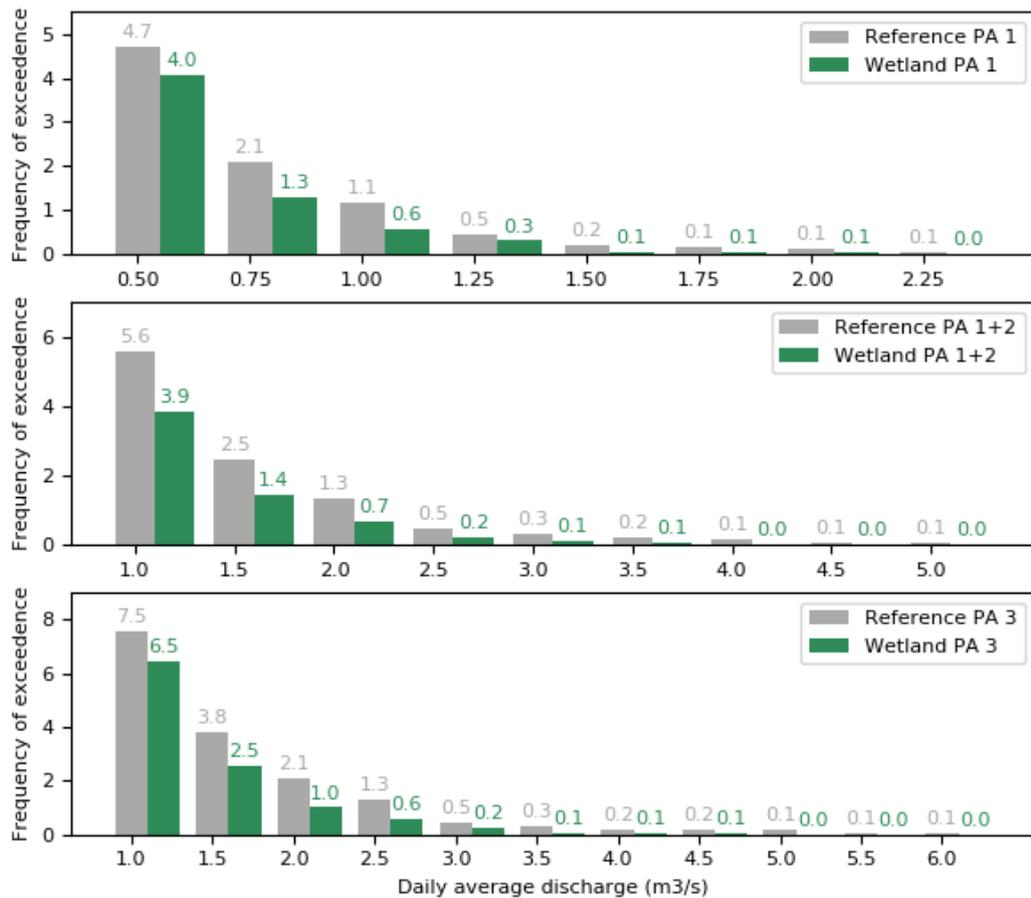
Figure 22. The average annual exceedance frequency of various winter peak flow rates in each of the three project areas under the reference situation and the wetland scenario (PA = project area).
