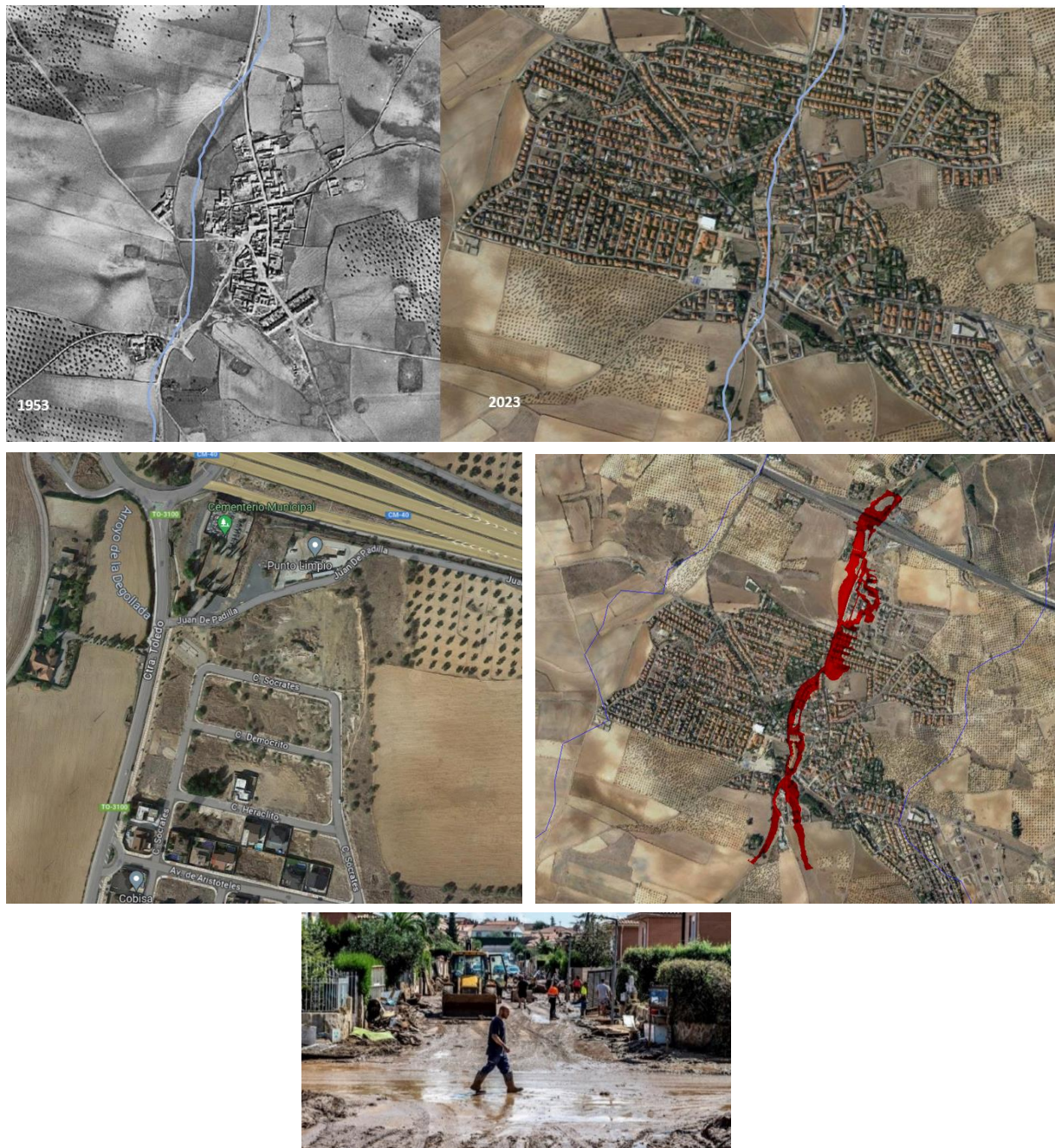
Figure 8: The expansion of Cobisa in the past decades on top of the streambed (upper photos). The expansion continues as new houses are built within the course of the Arroyo de la Degollada (lower left). Flood zones in Cobisa with a 500 year return period (lower right). Water filled with sediments flowed through the village of Cobisa on 3 September (below).
