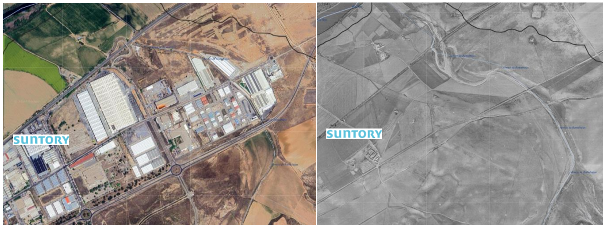
Figure 51: Location of the Suntory factory in the industrial site, with the Ramabujas canalised (left). The same location on the aerial photo of 1956, the Ramabujas at that time followed a natural course and had more space to handle high water discharges (right)
