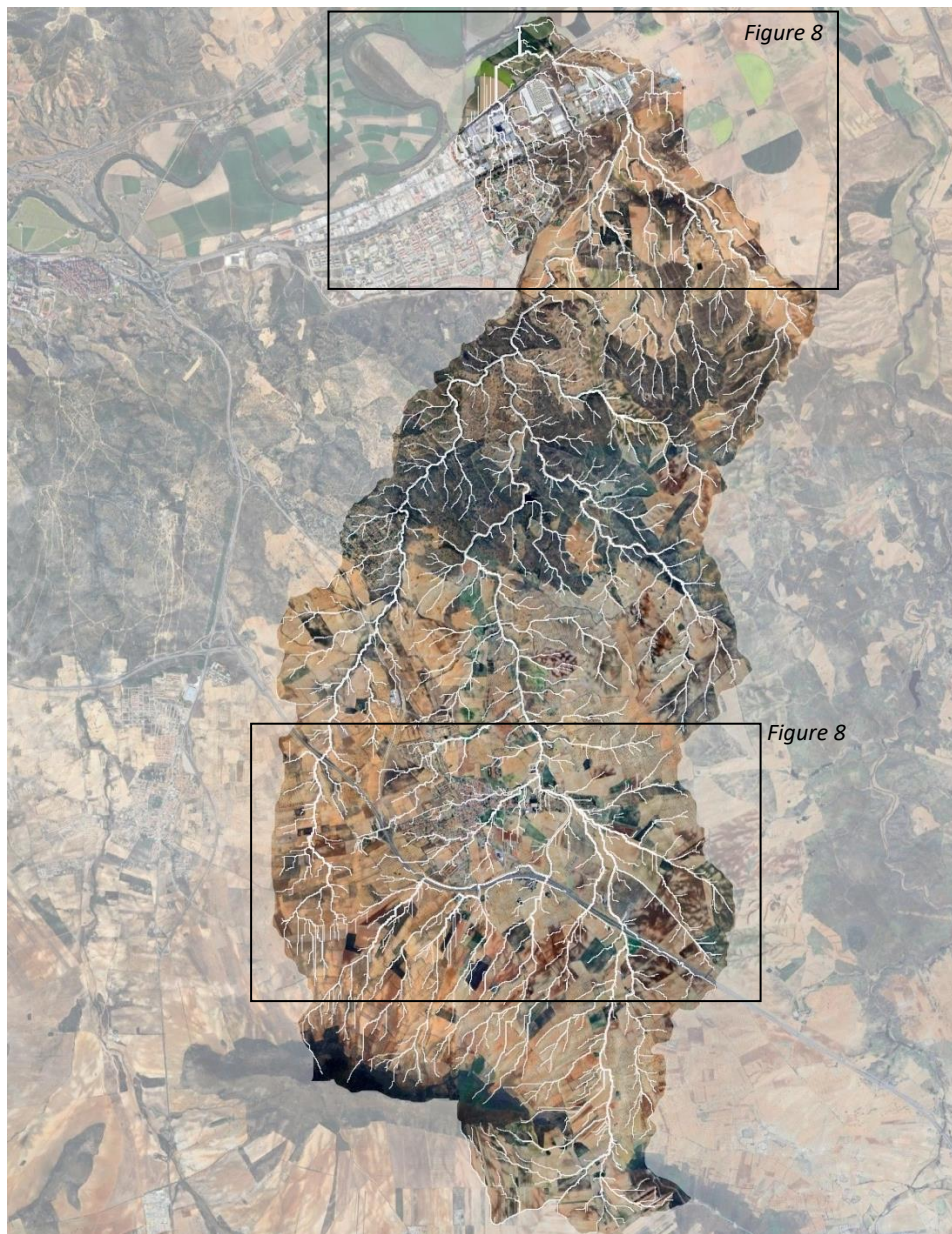
Figure 7: Drainage network of the Ramabujas stream catchment derived from 10-m DEM.
