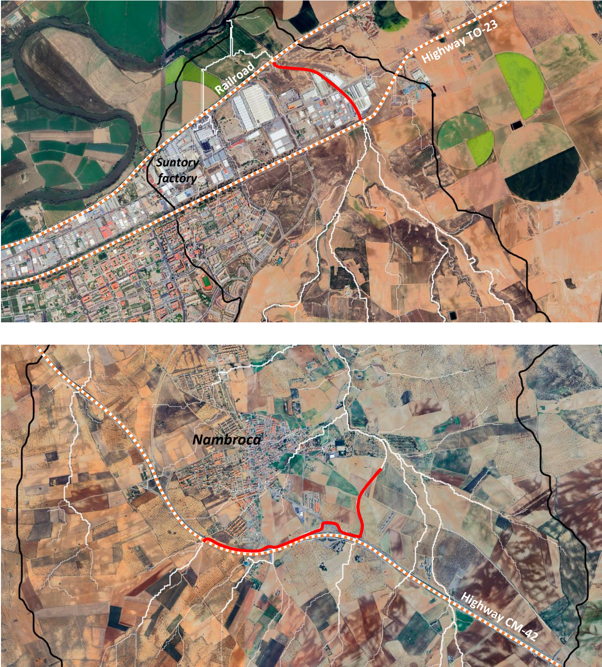
Figure 8: Culverts (where drainage lines cross the railroad and two highways) and artificial canals (red lines) in the industrial area of Santa María de Benquerencia (top), and around the village of Nambroca (bottom).
