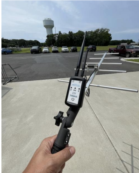
Picture 5. Image of the CTT Sidekick with the 2.4 GHz omnidirectional antenna, the 434 MHz omnidirectional antenna, and a Yagi antenna (with handle and connecting cable). More details: https://celltracktech.com/collections/digital-radio-products/products/ctt-sidekick
