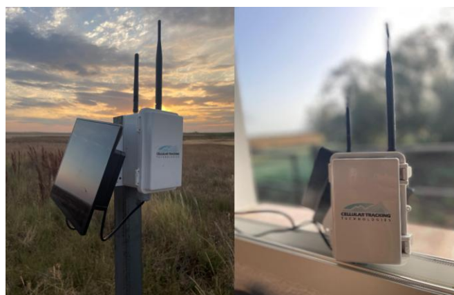
Picture 3. Pictures of the CTT Node V3. The system is powered by solar energy generated by a small solar panel attached to the node. Once assembled, it is only necessary to switch on the solar panel for the node to begin operating. More details: https://celltracktech.com/products/ctt-node%E2%84%A2-version-3-0-with-dual-radios-434mhz-and-2-4ghz?_pos=1&_sid=f7117fb6f&_ss=r&variant=50012198469792
