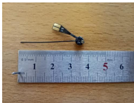
Picture 1. Photograph of the CTT BlūBat tag showing the test pad that must be cut before deployment on the bird to activate transmission. More details are provided at https://celltracktech.com/products/ctt-blubat?_pos=1&_sid=5c1e43853&_ss=r and the text below.
