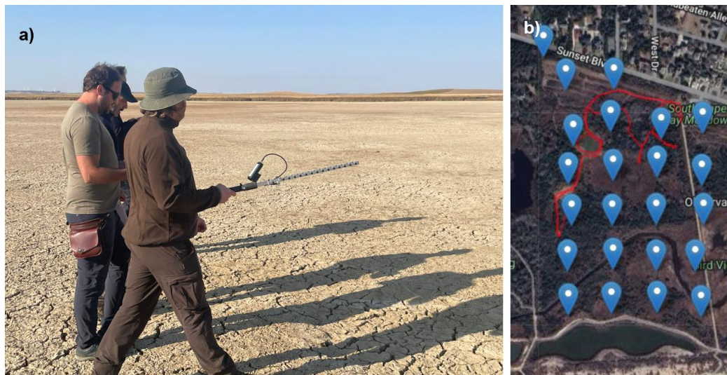
Picture 13. Walk-through calibration survey (a) carrying the Sidekick and an activated tag among the installed nodes (b).
