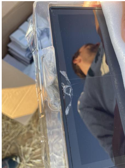
Picture 8. Broken solar panel in one of the nodes delivered for installation in Boada (Palencia).
