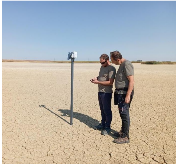
Picture 11. Temporary installation of one of the nodes to determine the detection range of the tags.
